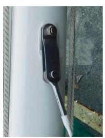
The end of the shrouds that connect to the shroud adjuster has been ground down to fit the thru-deck fitting. Larger, oversized aircraft eyes are used for strength. Sometimes the aircraft eyes are not ground enough for a particular boat. Simple put the aircraft eye on a grinder or use a file to get the correct fit. Sometimes, simply rounding over the aircraft eye will allow it to slide through the hole in the deck.
